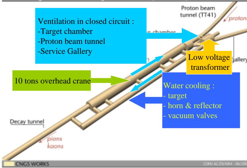
CNGS underground structures - hadron stop / muon detector area (not to scale)
