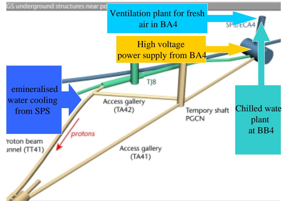
CNGS underground structures - target chamber area (not to scale)
