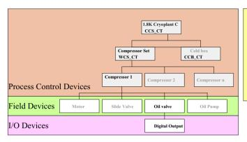
For each object type an adapted user interface is created & implemented in the supervision to allow monitoring & control
